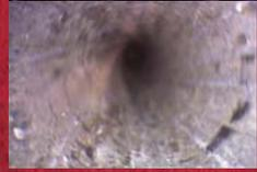
Bore scope photo of muzzleloader breech using Remington® Kleanbore® primers after 15 shots.
