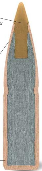
Thicker mid-jacket and heavy base for progressive expansion and maximum weight retention
