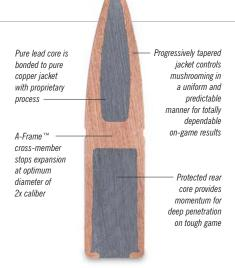
THE COMBINATION OF A-FRAME™ CONSTRUCTION AND PROPRIETARY BONDING PROCESS PRODUCES EXTREMELY UNIFORM, CONTROLLED EXPANSION TO 2X CALIBER WITH NEARLY 95% WEIGHT RETENTION.
