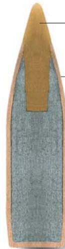
Gold polymer tip acts as a wedge, splintering bullet into fragments at impact
